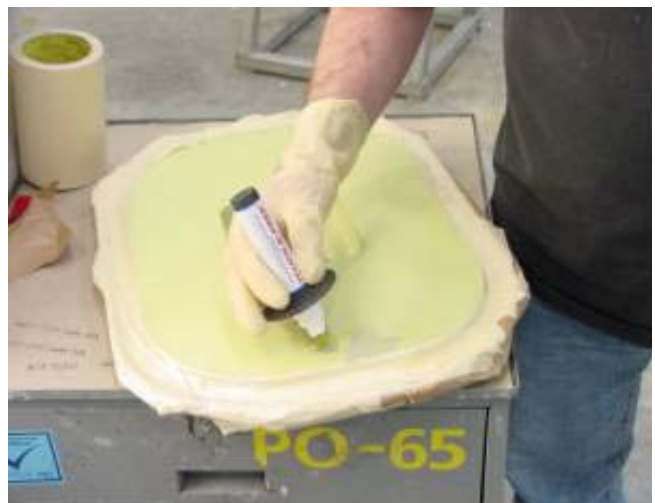
Figure 2 - Applying Alodine 1132 with Touch-N-Prep Pen to Restore Coating on Repair Area
